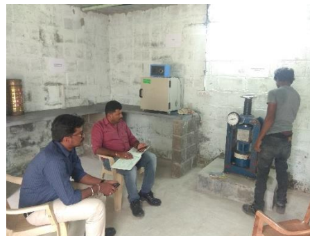
SIC Muralidhar G B along with Contractor's Engineer checking the crushing strength of concrete cubes.
